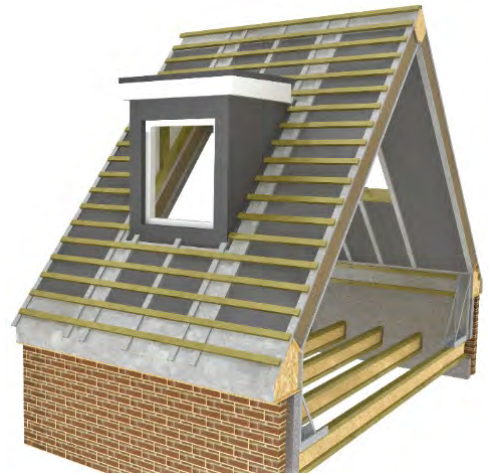
Roof with Dormer Fitted
