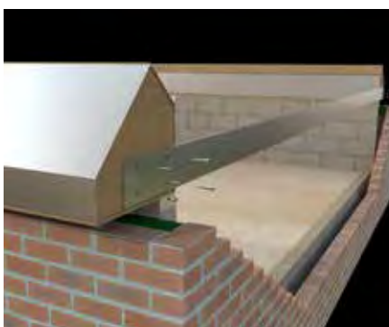
5. Secure each end of the tie plates with 3 x M10 x 25mm steel bolts and 2 x M10 coach bolts.
