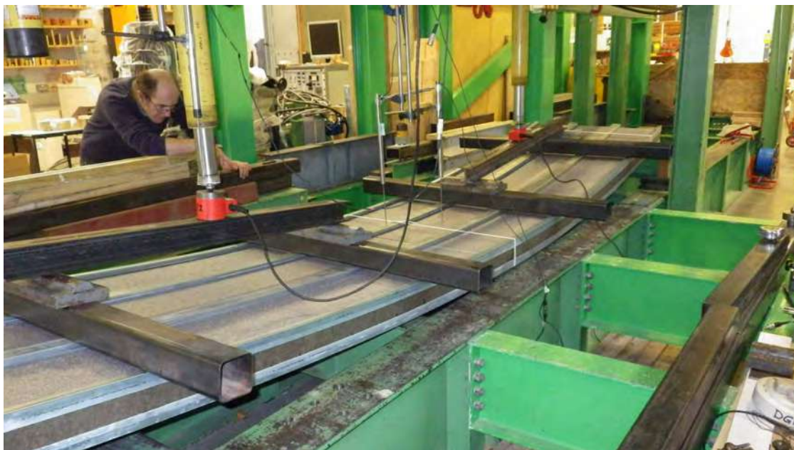
Figure 1.11 Deflection of 113 mm deep panel
