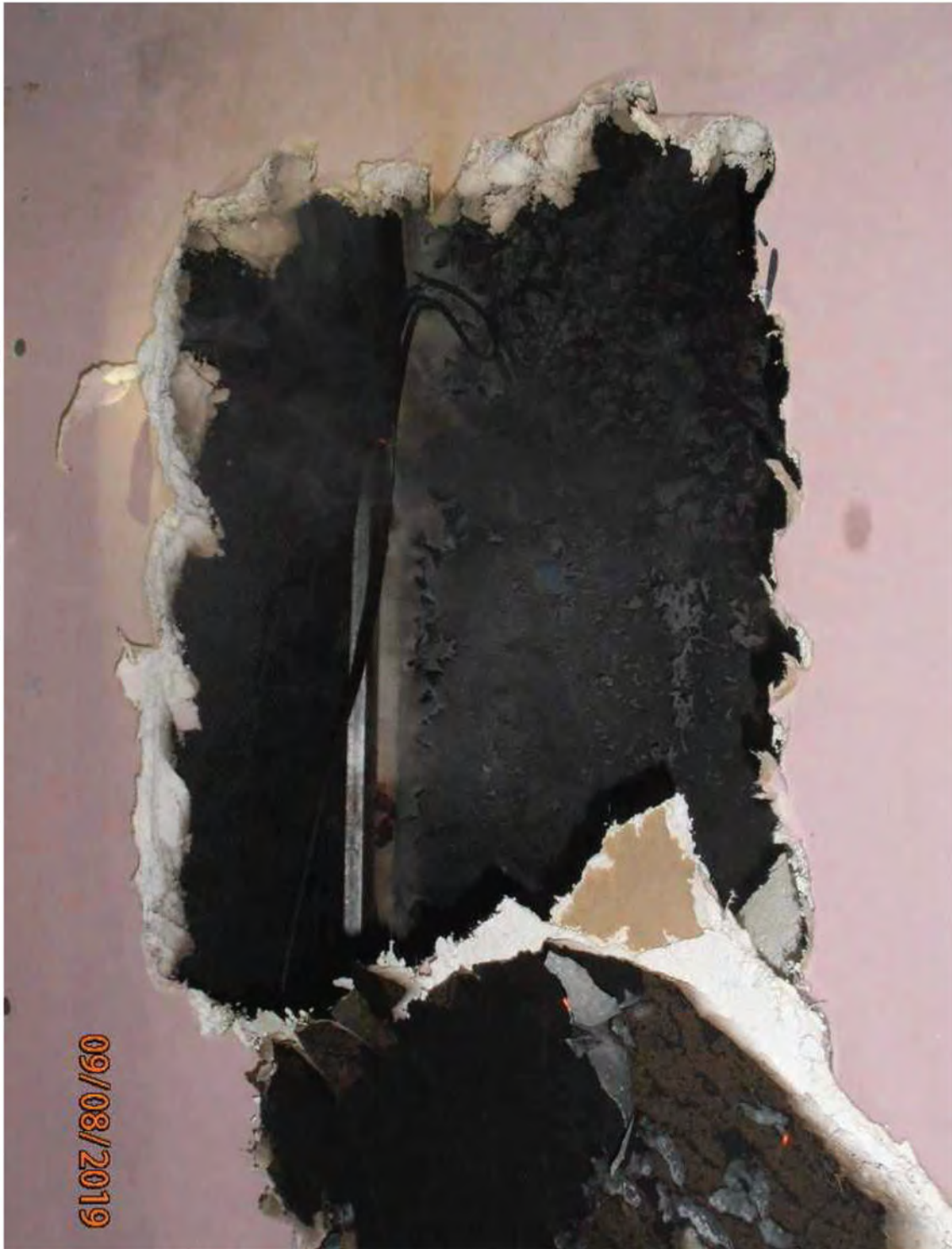
Photograph 15: View of internal wall cavity after test – from the unexposed face.
