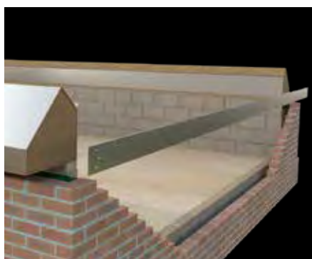
4. Support and offer up the assembled steel tie plate.
