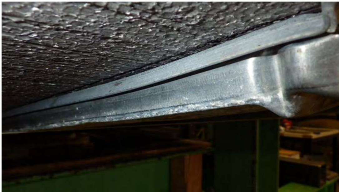
Figure 1.8 Local buckling – 213 mm deep panel
