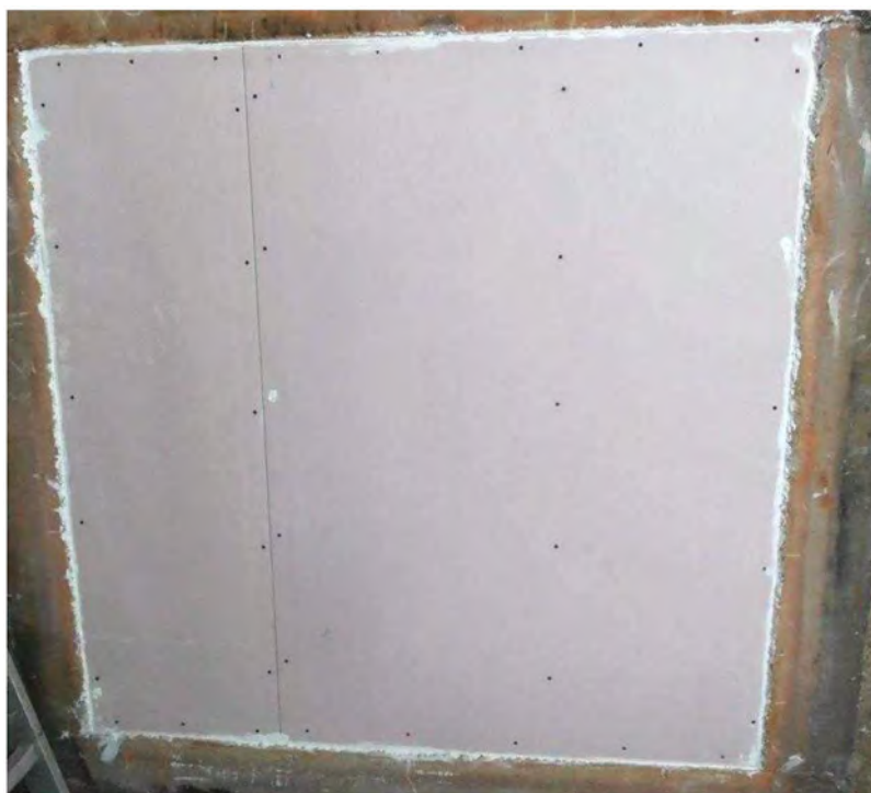
Photograph 7: Exposed face of Ultrapanel wall - after installation of 2 nd (outer) layer of plasterboard and prior to the start of the test.
