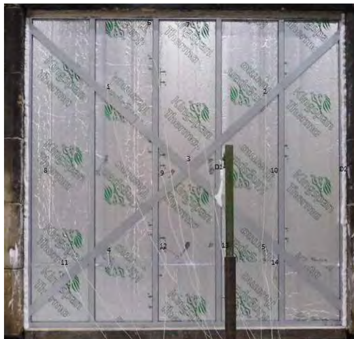
Photograph 1: Unexposed face of test specimen before test showing thermocouple and deflection locations.
