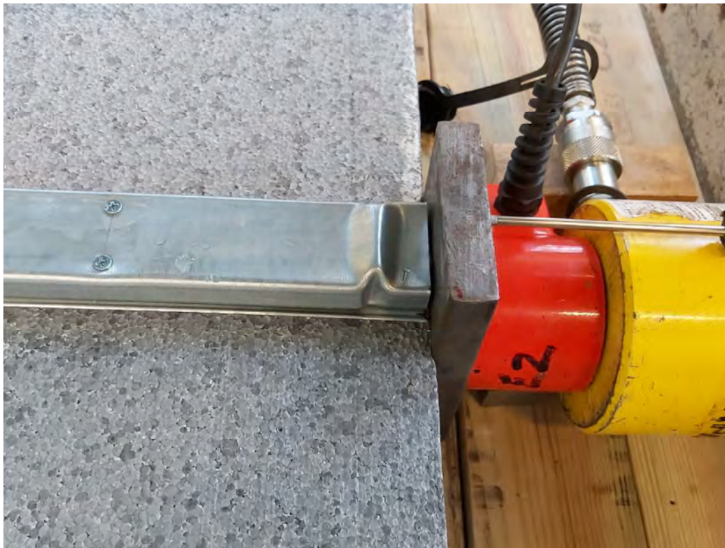
Figure 1.4 Buckling of steel 'flange' at end of member
