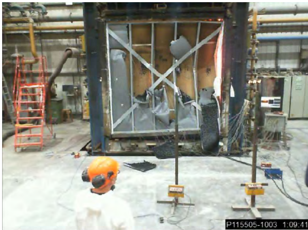
Photograph 4: Unexposed face of test specimen at point of loadbearing failure after 69 completed minutes of test
