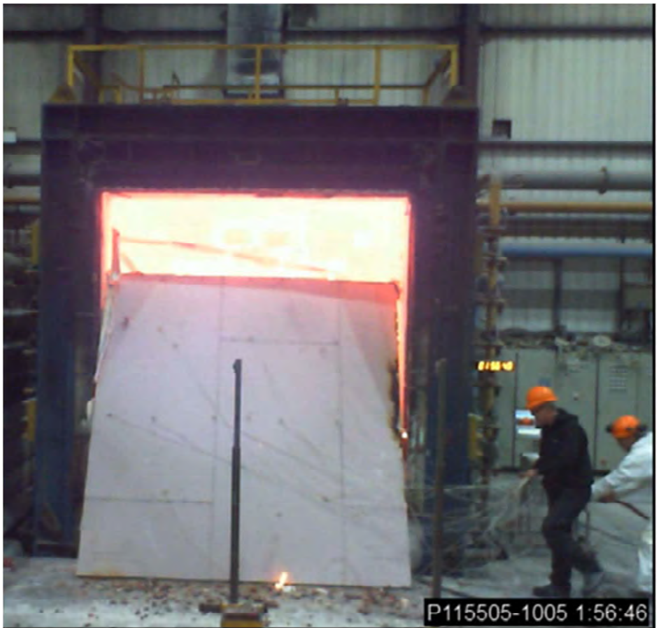
Photograph 5: Unexposed face of test specimen after the specimen jumped off the front of the furnace at termination of the test
