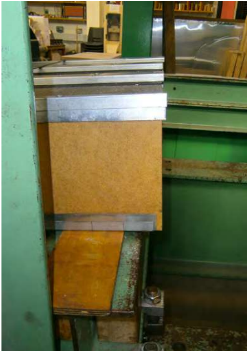
Figure 2.3 Permanent slip at ultimate load
