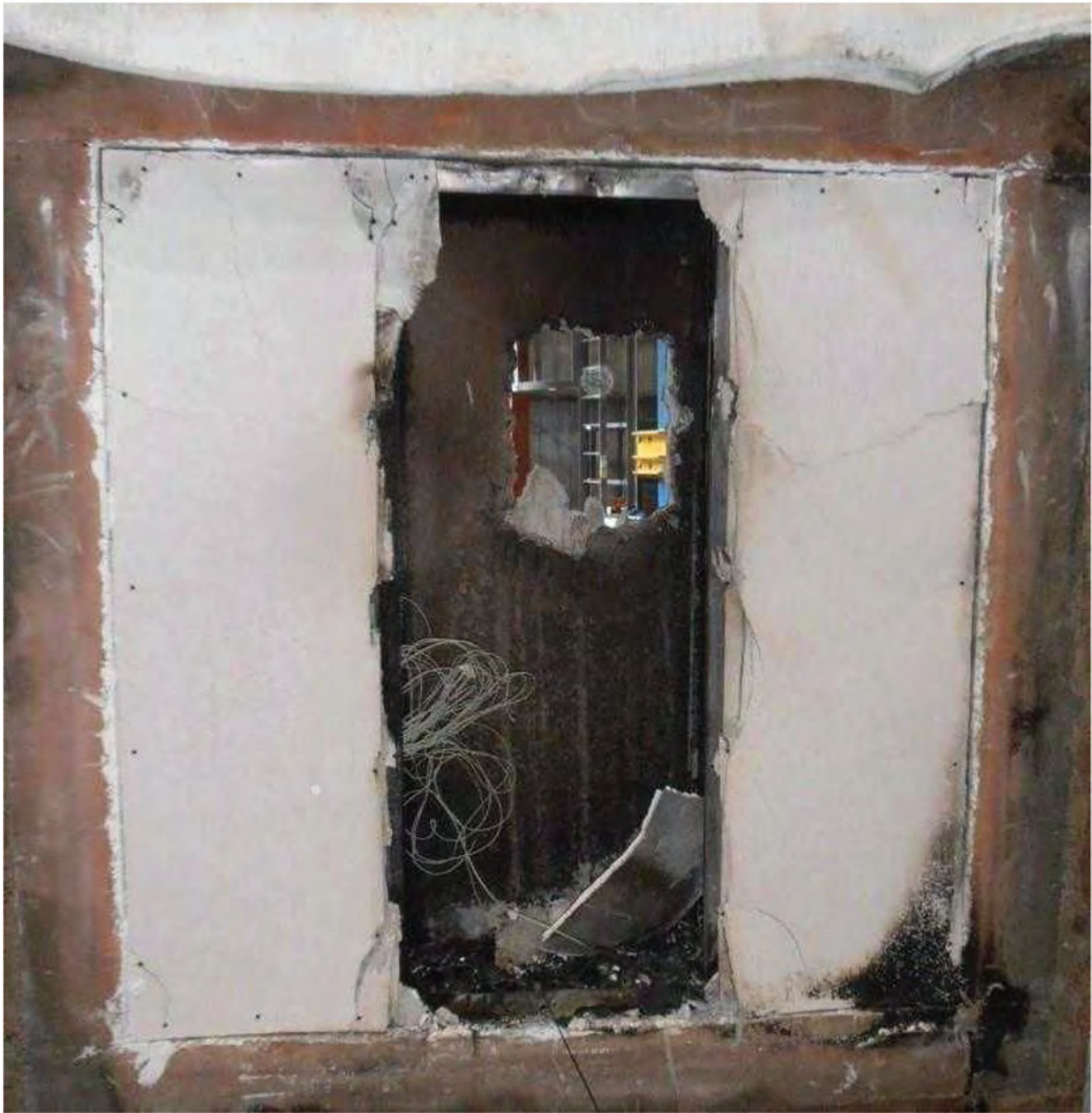
Photograph 16: Exposed face view of Ultrapanel wall - after test.
