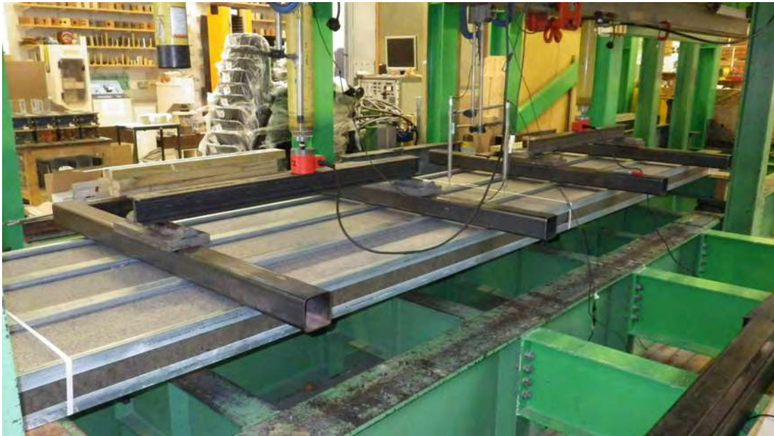
Figure 1.9 General arrangement of 113 mm deep panel bending tests
