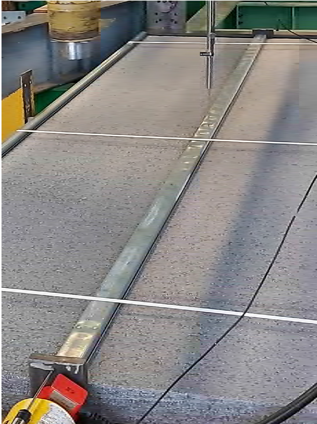
Figure 1.3 Local buckling of steel cover strip
