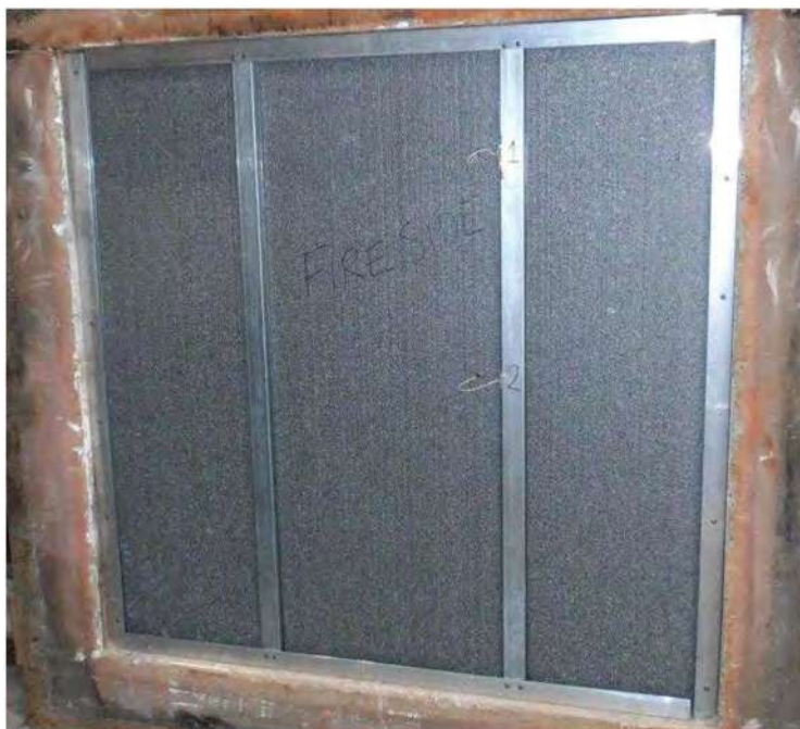
Photograph 4: Exposed face of view of Ultrapanel wall – showing installation locations of thermocouples 1 & 2.
