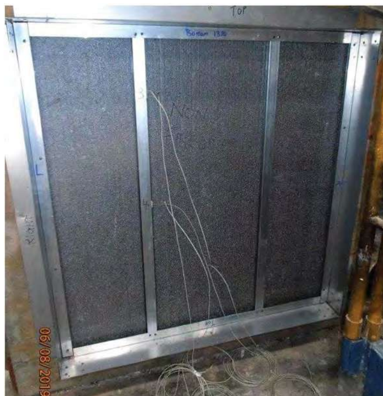
Photograph 5: Unexposed face of view of Ultrapanel wall – showing installation locations of thermocouples 3 & 4.
