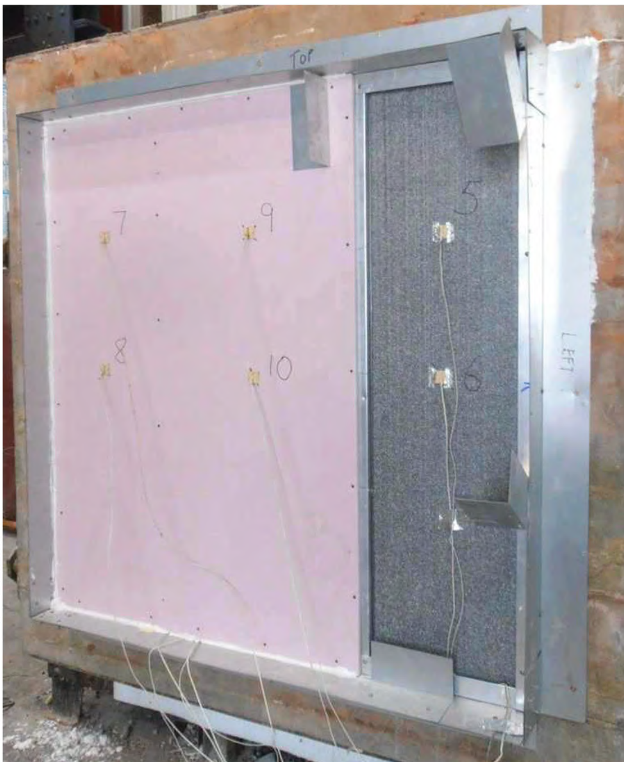
Photograph 8: Unexposed face of Ultrapanel wall – before the start of the test (with location of thermocouples 5 – 10 shown attached to the specimen).
