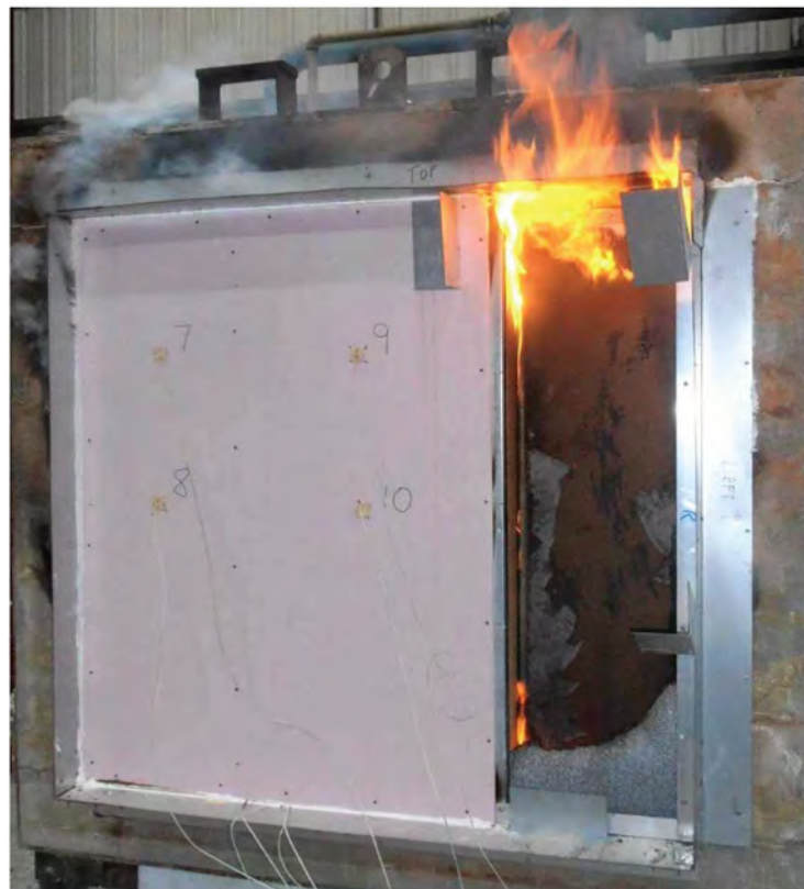
Photograph 14: Unexposed face of Ultrapanel wall – 115 minutes after the start of the test (immediately prior to test termination).
